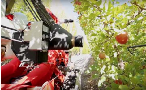
Abundant Robotics: a vacuum apparatus harvests mature apples from trees based on computer vision
