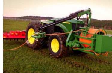
John Deere has developed a high-performance, autonomous, fully electric tractor.
